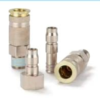
Industrial coupling with Atlas Copco-Profile. Coupling system with single-hand operation. High Flow valve for optimum flow and low pressure drop. Optimal for use with large pneumatic consumers due to the robust design and steel sleeve. The collar design minimises damage to the valve body.
