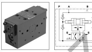
At the end of the intensifier's piston stroke, the rocker mechanism switches the directional slide valve to the crossed switching position, and the intensifier piston pumps oil from the piston rod area into the high pressure section. The process repeats itself until the pressure ratio corresponding to the surface ratio has lead to a balance of force on the intensifier piston.
