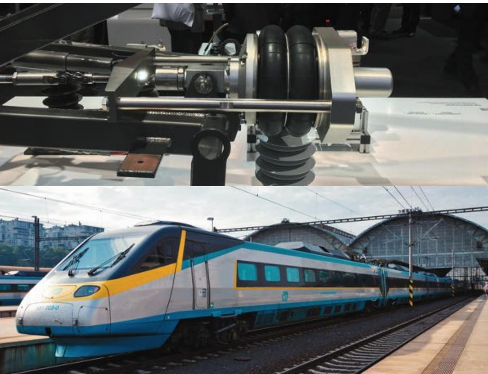
THE BELLOWS SPRING TYPE IS INTENDED FOR ELASTIC BEARING OF MACHINES AND INSTRUMENTS, TO ELIMINATE VIBRATIONS AND IMPACTS AND, ON THE CONTRARY, TO GENERATE VIBRATIONS AND LIFT OBJECTS. IN GENERAL, IT IS ABLE TO CARRY OUT WORK BY A DEFINED FORCE ALONG A DEFINED TRAVEL - see basic technical parameters.
