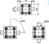
Available for P1F Profile and Tie-Rods versions the MT4 centre trunnion when combined with AT4 pivot brackets is intended for articulated mounting of the cylinder. The trunnion is free so that it can be fixed afterward when the cylinder is at the right place on the machine.
