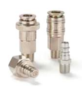
robust design (steel sleeve) and long service life even with the harshest use. Additional safety locking system. This safety lock prevents unintentional disconnection. To disconnect, the plug must first be pushed further into the coupling before it can be unlocked. The brass version has been developed specifically for use with water in the pressure range up to 35 bar.
