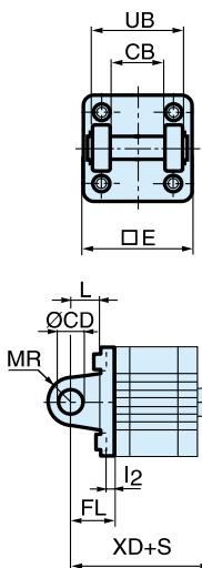
**Compact ISO Cylinders - P1P Series****Dimensions****Cylinder mountings****Clevis bracket MP4**
