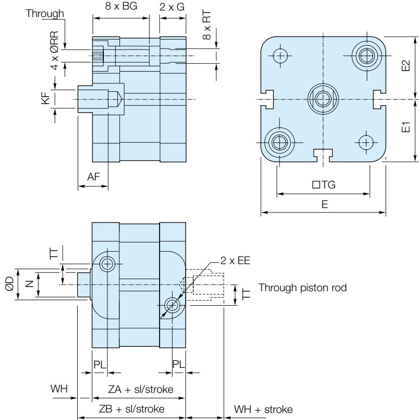
**P1PG...DS Double acting with guided piston rod**
