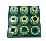
**QDC 239 B** Crimper die rack in front of machine for 9 sets\*
