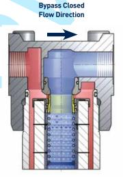
across the filter element. During bypass only a part of the main flow is flowing through the bypass valve.
