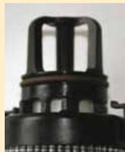
A new patented design of the filter element allows integration of the bypass valve and element core as re-usable parts in the filter bowl. This results in cost reduction when integrating the high pressure filter in manifold type solutions. But it also reduces the waste when changing the filter element by over 50% as the element core is an integral part of the filter bowl.
