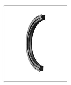
The profile BU Ultrathan® rod seal is a compact seal with an integrated antiextrusion ring. A typical application of this seal profile is its use as a buffer seal in sealing systems (picture) often found on construction machinery cylinders. These cylinders operate under extreme conditions where pressures up to 1000 bar are not unusual.
