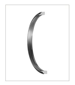
The function of the profile A1 Ultrathan<sup>®</sup> wiper ring is to prevent dust, dirt, grains of sand and metal swarf from penetrating. This is achieved by a special design which largely prevents the development of chamfers, protects the guiding parts and extends the working life of the seals.
